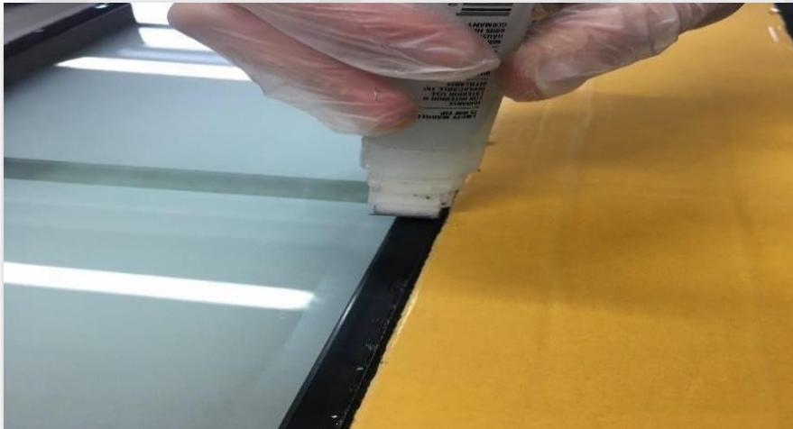
After the entire preparation process for gluing the overlay panels (the process described in paragraphs above), remove the protective layer from the tape just before gluing the internal part.
