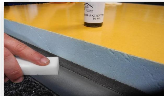
After activation of the aluminium, apply SIKA PRIMER 206G+P on the glued components, carefully, so other components of the panel or the leaf are not contaminated.
