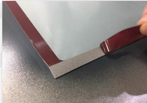
After the internal metal sheet is glued together with other components of the structure, press the glued surface evenly and strongly.
